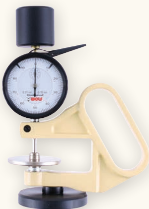
DMH 3-L especially for leather with a standardised gauging pressure of 50 kPa
